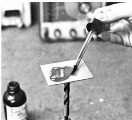
fig. 11. A thin, even coat of photoresist is applied to the board by spinning it with a drill motor.
